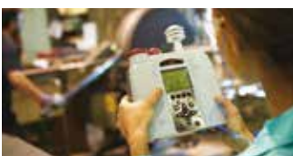
3M™ EVM Monitors measure hazards in real-time
